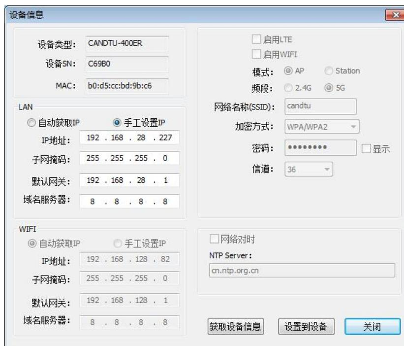
Figure 4.4 Device network configuration 2
